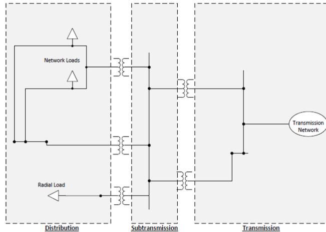
**Figure 1. Typical Electrical System**
