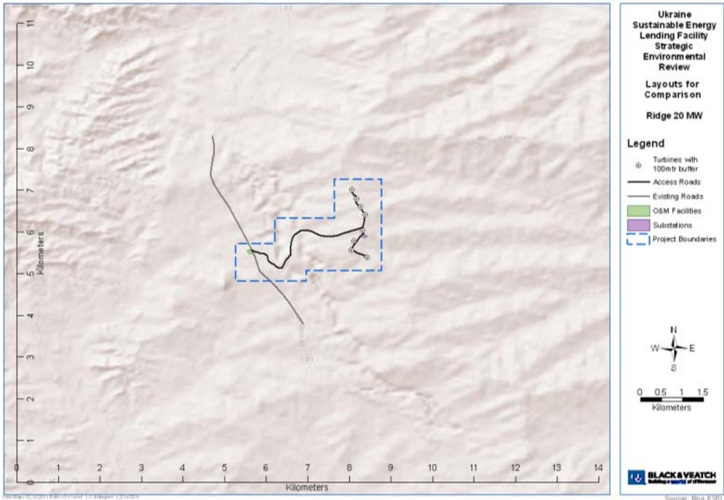
**Figure 3-9. Representative Project Configuration (20 MW) on Ridgeline.**
