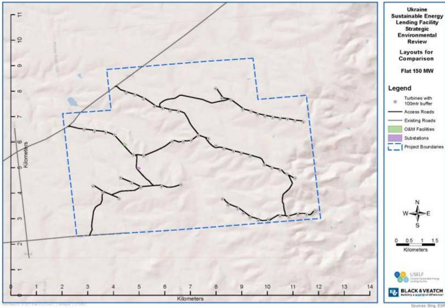
Figure 3-8. Representative Project Configuration (150 MW) on Flat Land.
