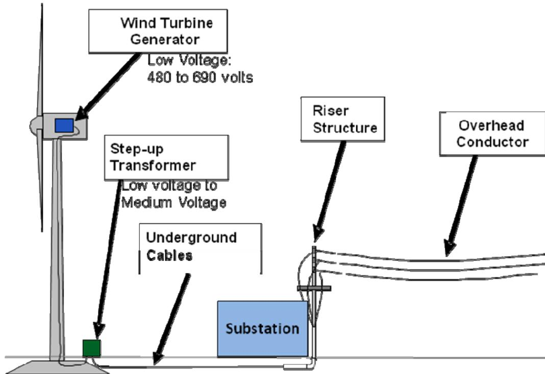
Figure 3-3. Typical Wind Collection System Arrangement.
