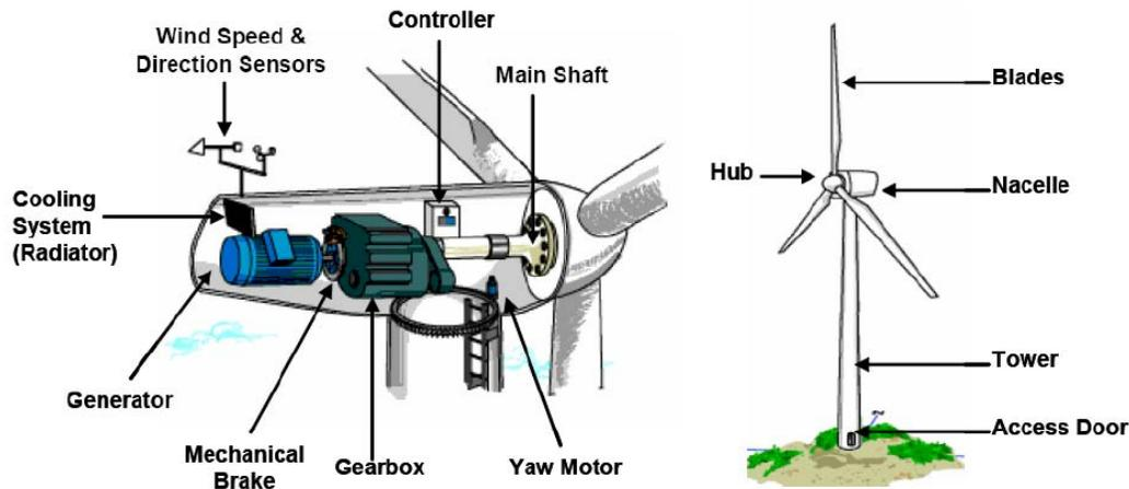
Figure 3-1. Typical Wind Turbine Schematic.
