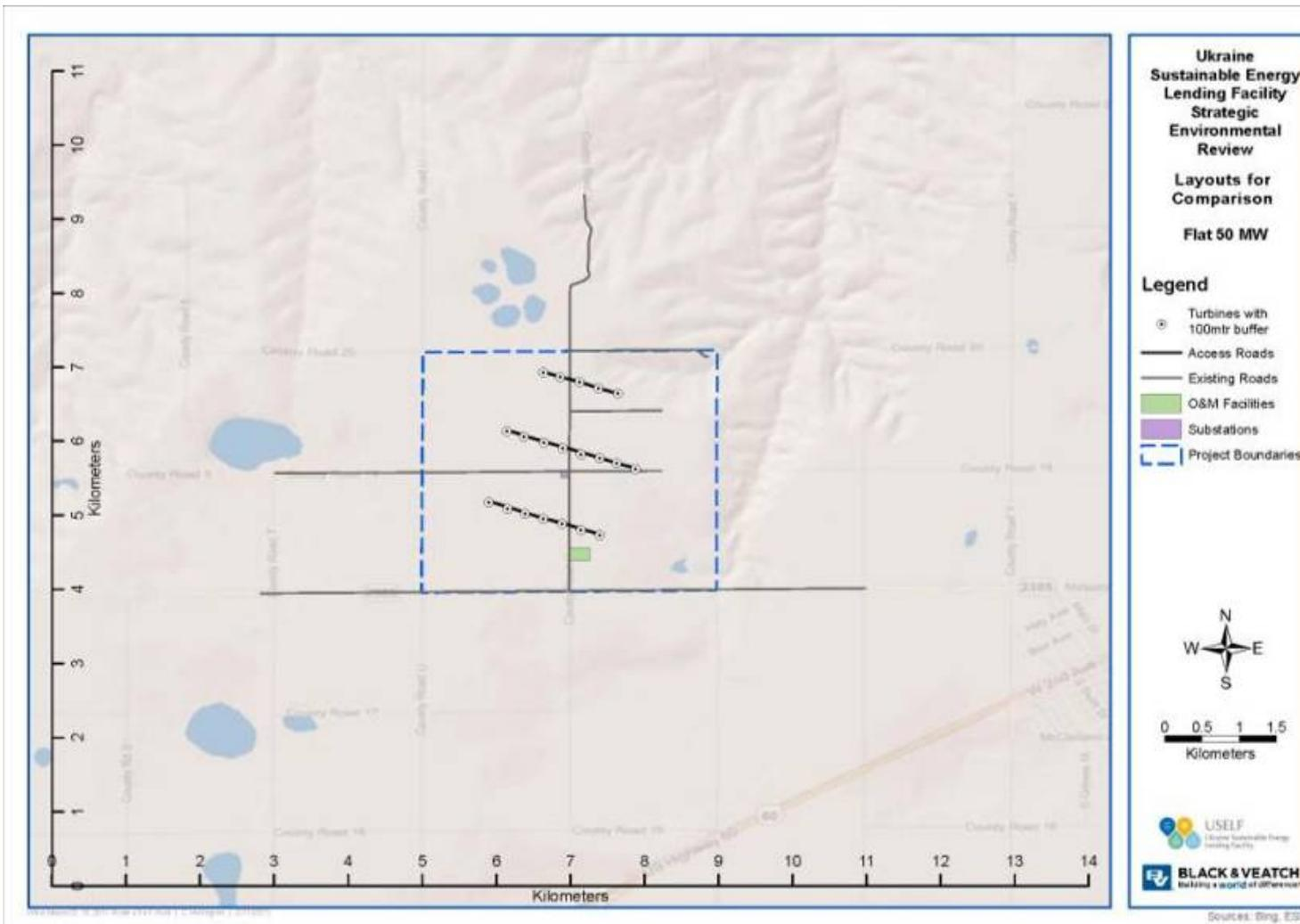
Figure 3-7. Representative Project Configuration (50 MW) on Flat Land.
